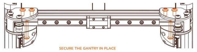
Now we can tighten the 6 screws we left loose earlier. This will complete the installation of the gantry.
